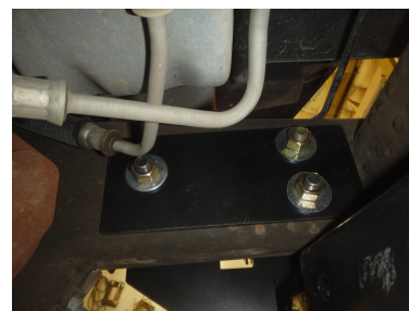
Inner frame plate and fasteners
