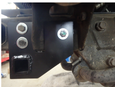
Receiver/frame mounting detail
